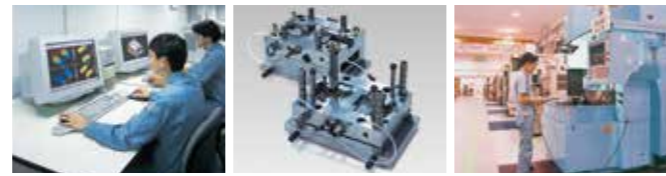
● Design with 3-D CAD ● Manufacturing of metal molding parts ● Electrical discharge machine
